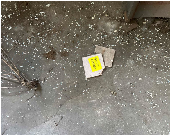
Line ID 16: Internal, GF, Old Mortuary, South Room, on Floor, Fibre Cement Sheetting - No Asbestos Detected
