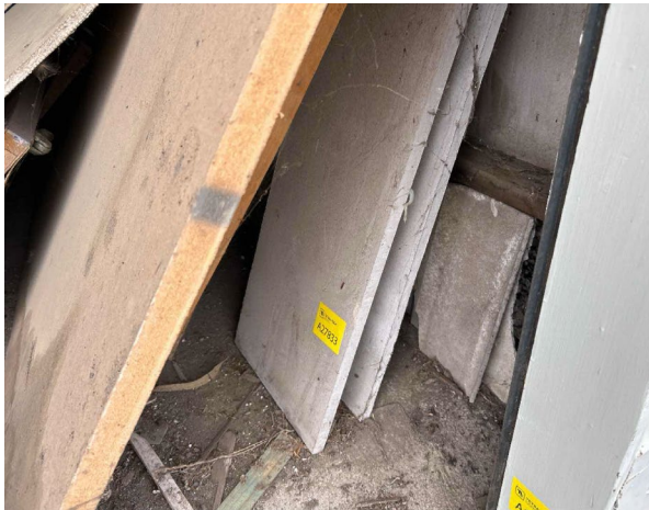
Line ID 29: Internal, GF, Workshops, Southern Section, Unit 1008, Northeast, Stored Sheets, Compressed Cement Sheeting - No Asbestos Detected
