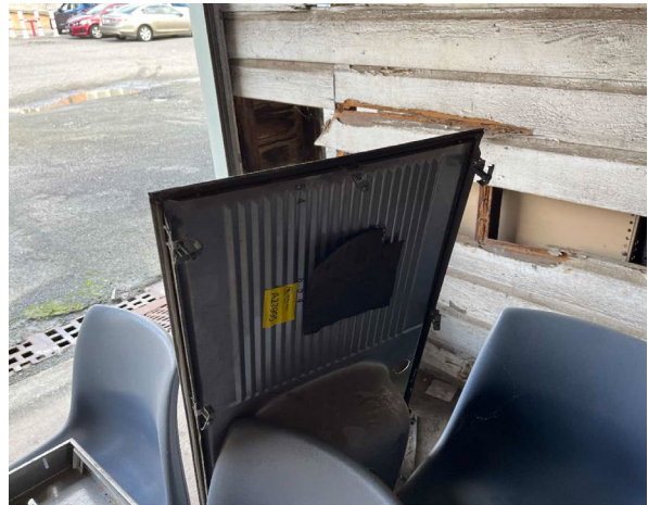
Line ID 32: Internal, GF, Workshops, Southern Section, Unit 1010, Stored Item, Underside of Sink, Bituminous Material - Chrysotile Asbestos Detected
