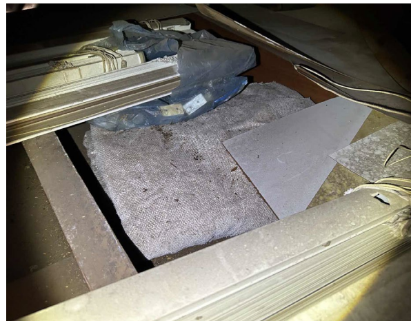
Line ID 19: Internal, GF, Workshops, Central Section, Ceiling Space, Adjacent Access Hatch, Woven Blanket Material - Chrysotile Asbestos Detected
