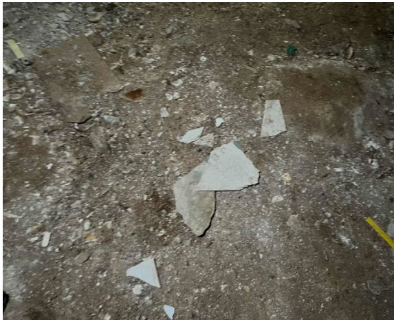
Line ID 24: Internal, Basement, Storage Area, Subfloor, Fibre Cement Debris - No Asbestos Detected
