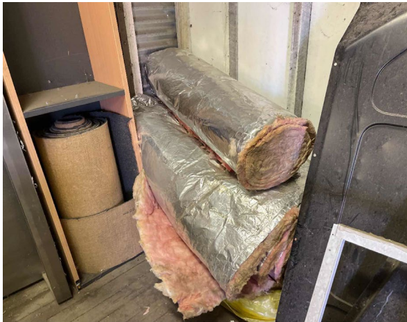
Line ID 52: Internal, GF, Workshops, Northern Section, Room 1004, Sarking Insulation, Stored Item - Suspected SMF
