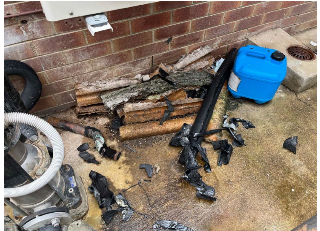
Line ID 131: External, GF, Central Wing, Central Alleyway, Pipework debris, Insulation Material - Suspected SMF
